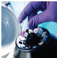
Figure 7.9 Separation of a solid from a liquid in a laboratory centrifuge
