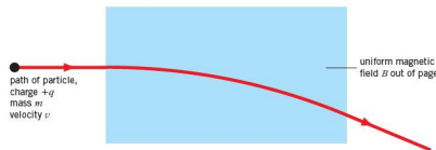
Figure 22.16 Path of a charged particle in a magnetic field
