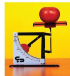
Figure 2.18 Lever balance with circular scale
