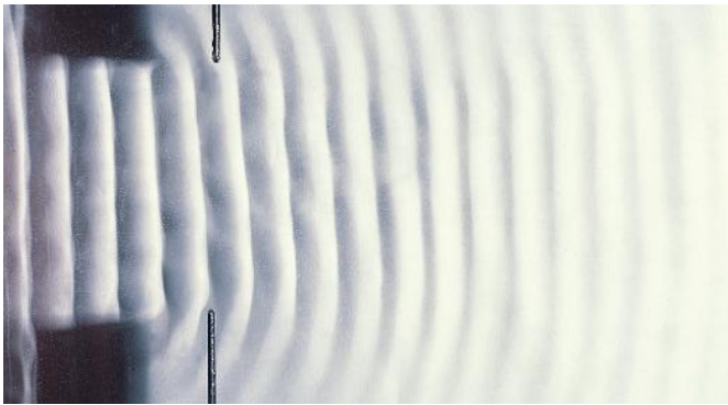
Figure 25.8b Spreading of waves after passing through a wide gap
