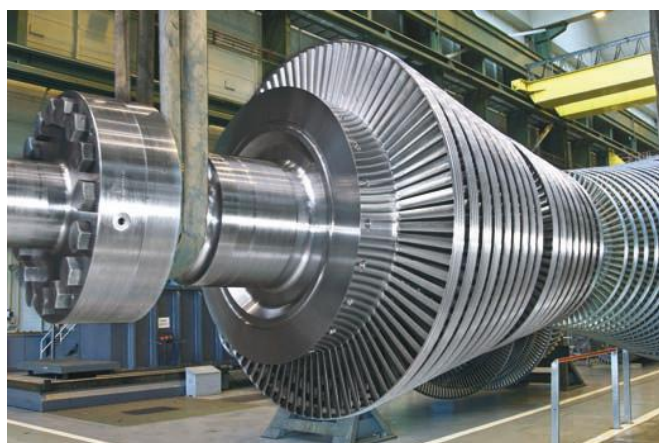
Figure 15.6 The rotor of a steam turbine
