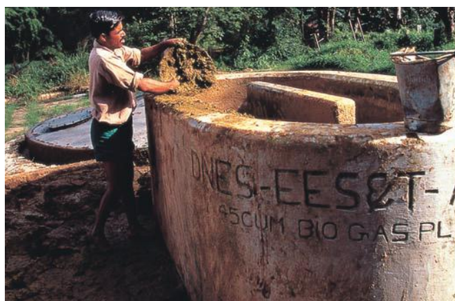
Figure 15.5 Feeding a biogas digester in rural India
