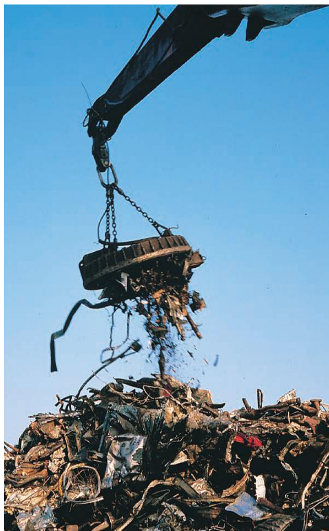
Figure 45.7 Electromagnet being used to lift scrap metal
