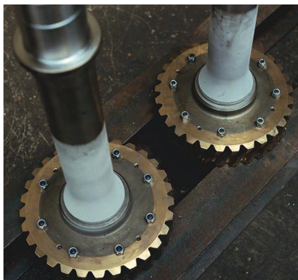
Figure 19.1 'Shrink-fitting' of axles into gear wheels
