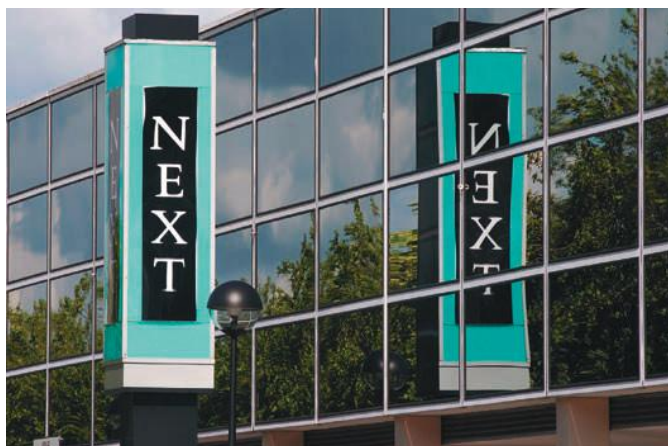
Figure 28.3 The image in a plane mirror is laterally inverted.
